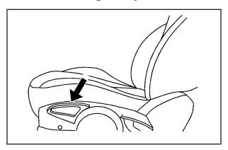
The driver's seat height adjuster is located on the outboard side of the seat.
